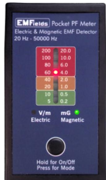
The easy-to-use Pocket PF5 meter measures magnetic *and* electric fields from power-frequency sources.
